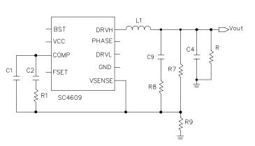
Figure 4. Compensation network provides 3 poles and 2 zeros.
