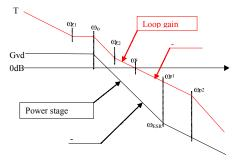
Figure 5. Asymptotic diagrams of power stage and its loop gain
