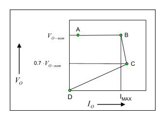
Figure 2. Over current protection characteristic of SC4609
